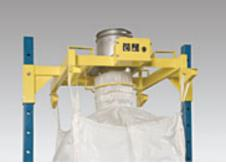
Flexicon's lowest cost bulk bag filler is a lighter duty version of the company's patented Twin-Centerpost™ design offering extreme structural integrity and easy access to bag connection points at minimum cost.
